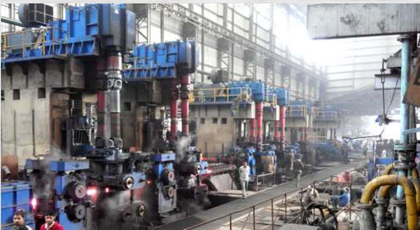
H – V Mill, Housing less Stands, for Stainless Steel Wire Rods 250,000 tpa
