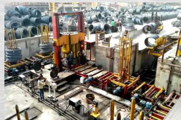
Vertical Coil Compactor, 2000 kg coil
