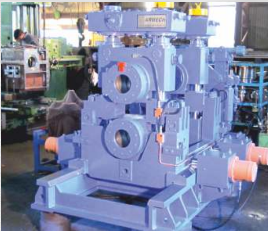
Housing Less Stands: Standard Roll Neck Sizes: 160 / 200 / 230 / 260 / 280 / 320 mm
