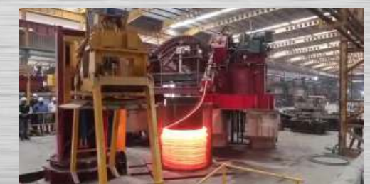
COIL BEING FORMED Rimjhim Ispat Ltd., Kanpur, India
