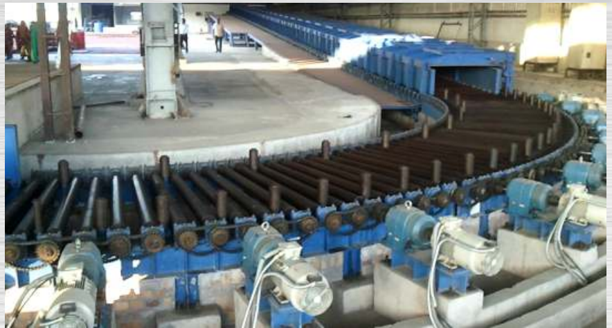
Controlled Cooling Conveyor with Insulated Covers for Low Carbon Grades
